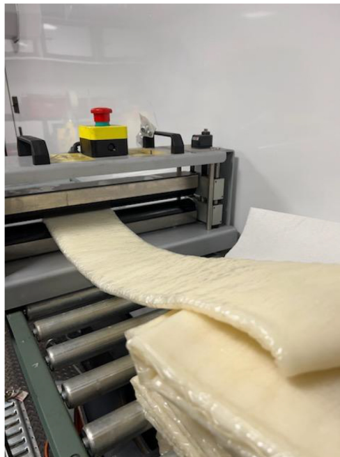
Calibrated, wet-out liner
