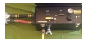
3. With the Air lever in the Off position attach the air hose from the compressor to the front of Heater Control Unit as shown. With the Heat switch in the Off position connect the power cable to the side of the Heater Control Unit as shown.
